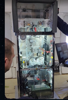
Metal foundry and continuous casting hardware for in-space operation
